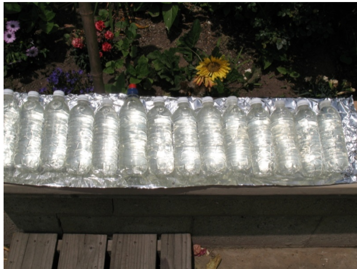
Figure 7 TRUSTED Filtered Water Is Exposed To The Sun For One Day (SODIS Method)
